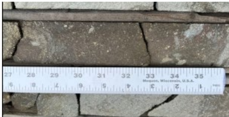
Allochthonous, brecciated massive sulfide hosted by Pipe Formation metapelite containing metapelite clasts, drill hole 102509
