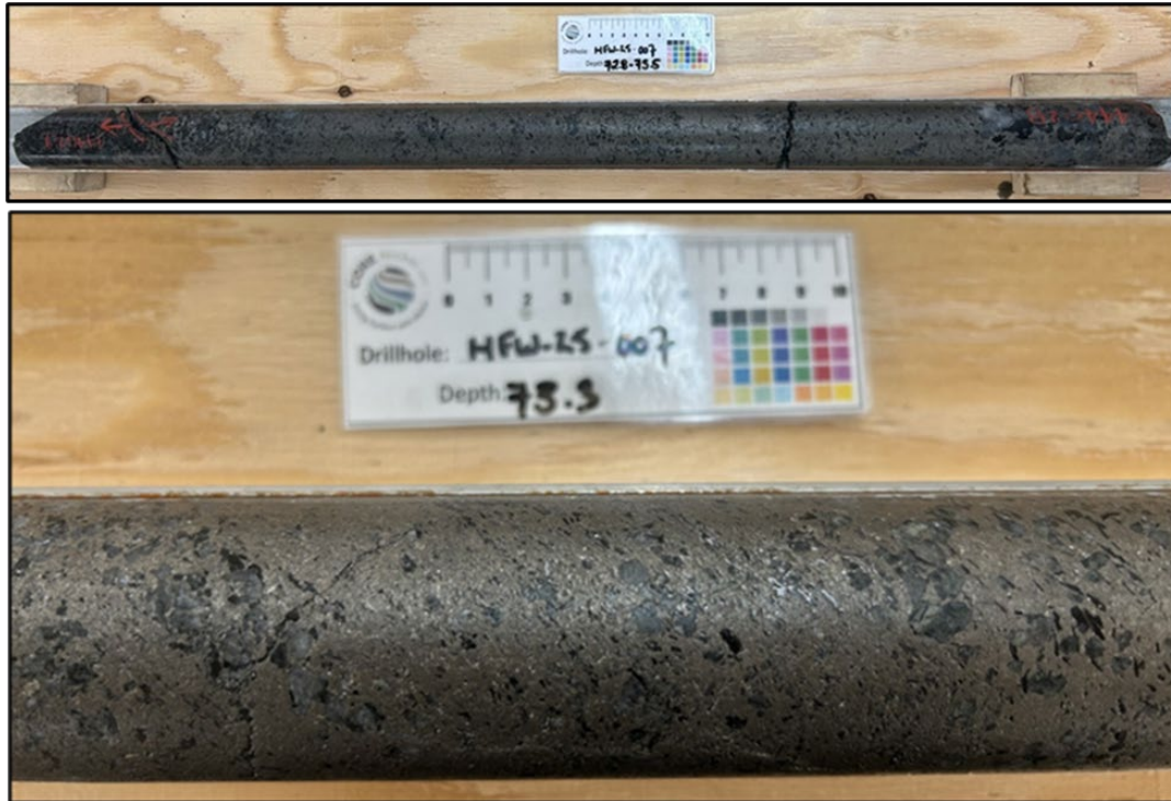
Figure 2. Top: Massive sulphides, dominantly pyrrhotite in HFW-25-007 from 72.8 to 73.5 m. Bottom: Close-up of massive sulphides at 73.3 m in HFW-25-007.
